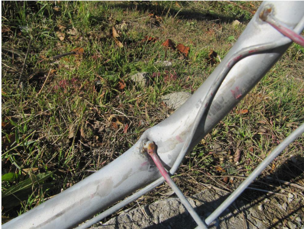
Figure 16: View of dark rubber transfers and burgandy paint tranfers indicating that contact was made by the SUV to the vertical post of the fence at the east edge of the hole.
