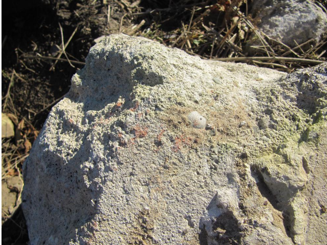
Figure 22: View of the reddish paint transfers on the concrete boulder confirming the SUV's impact with it.
