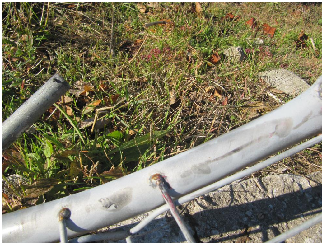
Figure 15: View of the dark transfers on the vertical post of the fence caused from contact by one of the right side tires of the SUV.
