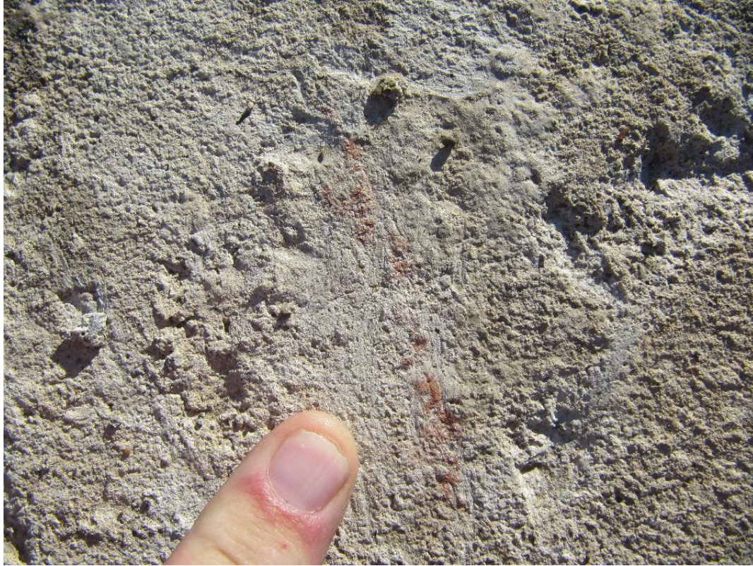
Figure 24: Close-up view of linear scrape and reddish paint transfers to a boulder that was struck by the SUV.
